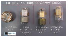
The quartz crystal oscillator utilizes the mechanical resonance from a vibrating crystal to create an electric signal with a very precise frequency. It is the source of radio frequencies and thus, the little gem behind the mass communication revolution that swept the 1930's and 1940's. Without the QCO, there would
